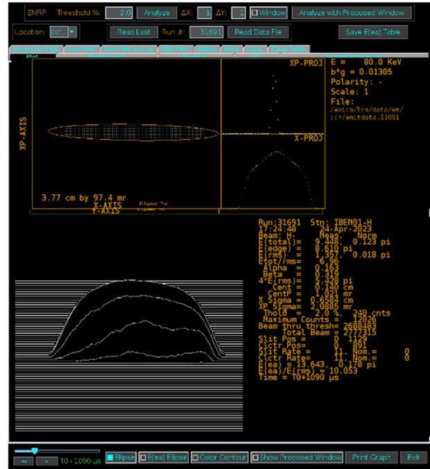
Figure 4: IBEM01 horizontal emittance scan.
