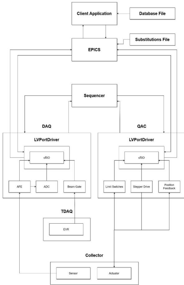
Figure 2: Emittance hardware block diagram.
