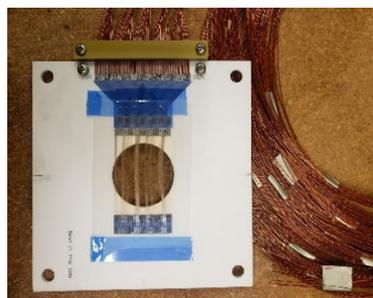
Figure 3: Wireplane with Kapton insulated signal wires.
