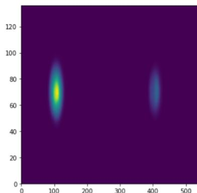
Figure 6: An example image from the CMOS camera when the bulbs are flashing. The light from the quartz rod is seen on the left and the capillary is shown on the right.
