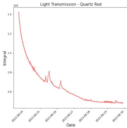
Figure 7: Light transmission of the quartz rod.
