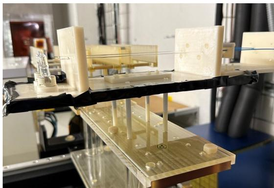
Figure 4: A quartz rod and EJ-309 capillary fibre installed at IRRAD. Two halogen bulbs are seen on the left and the transport fibres are seen on the right (blue cladding).
