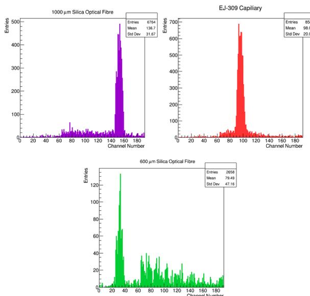
Figure 5: Beam profile measuring using 1000  $\mu\text{m}$  silica fibres (top left), EJ-309 capillaries (top right), 600  $\mu\text{m}$  silica fibres (bottom).
