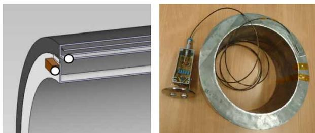
Figure 5: Alternative shielding geometry with axial meanders (left), the SQUID, housed in the little brown box, is connected between the two marked dots. Right: prototype of the Axial CCC made from Lead with attached SQUID electronics.
