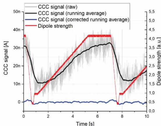
Figure 3: Effect of dipole ramp in CRYRING on CCC-XD measurement. Since the dipole ramp is deterministic it can be subtracted with an appropriate transfer function. The 1.4 Hz perturbation from the cryostat pulse tube cooler, visible on the raw signal, was eliminated by a software bandblock filter (1-3 Hz) [9].
