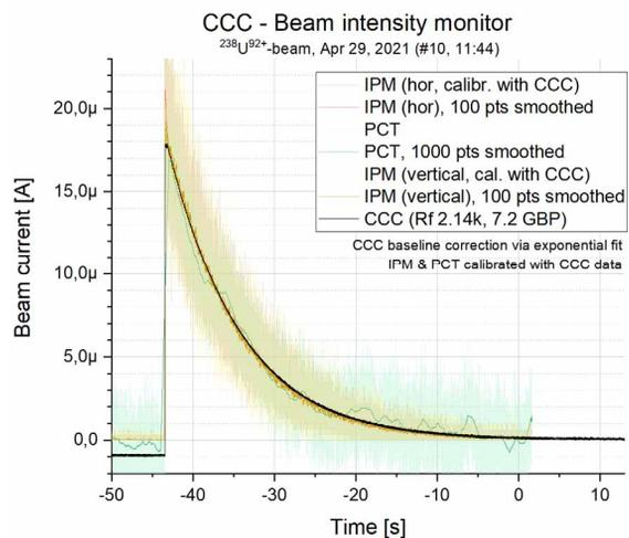
Figure 4: CCC current measurement compared to IPM and PCT in CRYRING. Rf = Feedback resistor value, GBP = Gain Bandwidth Product of the SQUID electronics [9].
