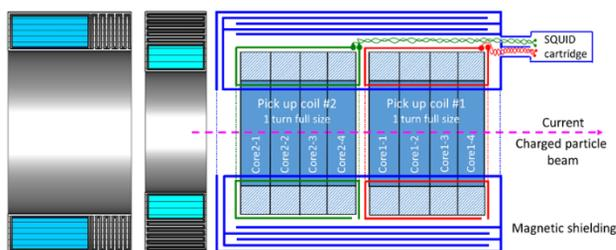
Figure 2: Magnetic shieldings with radial (left) and axial (middle) meanders. The ring-core of the radial CCC is indicated in blue, the detector volume of the axial CCC in turquoise. Right: Schematic sectional view of the DCCC with axial meanders and two independent, fourfold segmented (due to material width limitations) toroidal cores.
