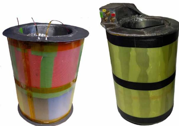
Figure 7: DCCC prototype, built from lead with diameter 300 mm and length 600 mm. Left: Pickup coils #1 and #2 mounted to the inner cylinder of the shielding (covered with tape). Right: DCCC completed and closed, with the outer meander shielding and the SQUID housing.
