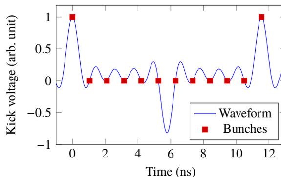
Figure 2: Kick action only on bunches at a bunch frequency equal to the fundamental of the kick waveform,  $f_{HK} = 86.6$  MHz; in this example, all 11 buckets are filled at a bunch frequency of  $11 f_{HK} = 952.6$  MHz.
