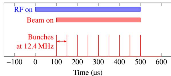
Figure 3: Macropulse timing for clean beam delivery while the cavity is on. Bunch spacing exaggerated for visual clarity.
