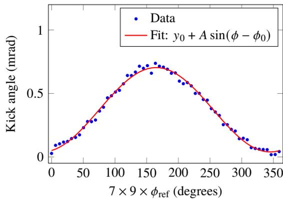
Figure 6: Deflection waveform with only the 9th harmonic (779.4 MHz) being driven at nominally 50 % output power. The phase  $\phi_{\text{ref}}$  being scanned is that of the 12.4 MHz reference and is scaled up accordingly for clarity. The beam angle is not explicitly corrected to give zero with the cavity off.  $y_0 = 0.372(3)$  mrad,  $\phi_0 = 75.1(7)^\circ$ ,  $A = 0.333(4)$  mrad.
