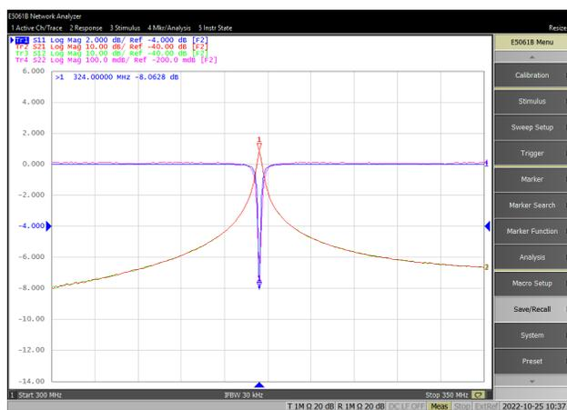
Figure 8: S-parameters of the prototype RF deflector measured by Keysight E5061B.
