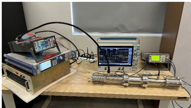
Figure 9: Tested by a 324 MHz power amplifier (Pmax=1 kW).
