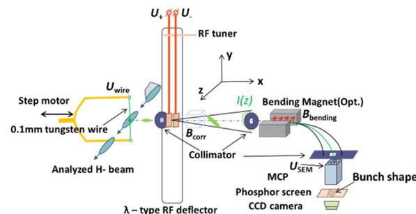
Figure 2: Configuration of bunch shape monitors in CSNS-II.
