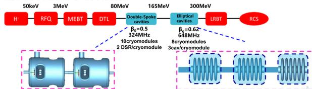
Figure 1: Superconducting cavities in CSNS-II [2].
