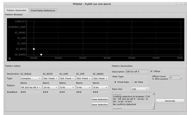
Figure 10: TPGGUI showing beam request with offset pulses between SC\_DIAG0 and SC\_BSYD.
