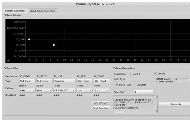
Figure 12: TPGUI showing beam request on offset pulses between SC\_HXR and SC\_SXR.
