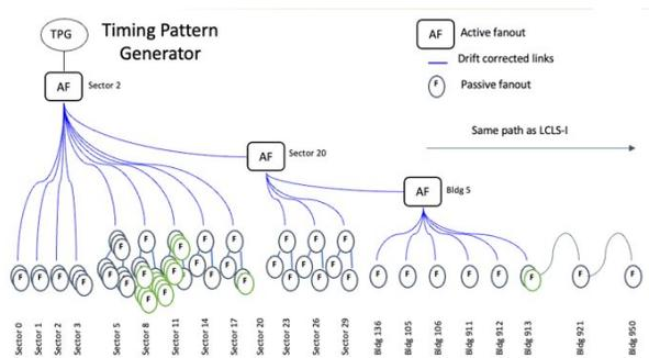
Figure 3: Timing fiber distribution.
