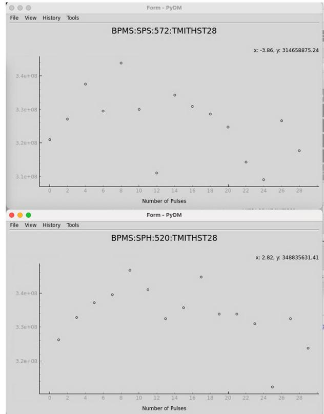
Figure 13: Beam pulses collected in the SC\_HXR and SC\_SXR areas at 1 Hz corresponding to the pattern shown in Fig. 12.
