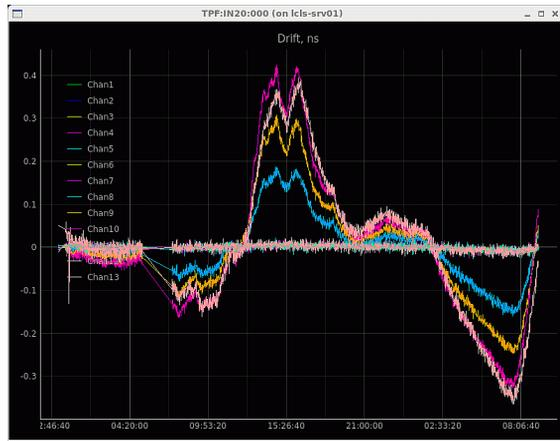
Figure 4: Signal drift on 6 channels measured at the Sector 20 Active Fanout. On the y axes the signal drift (1 ns) over time (about 12 h).
