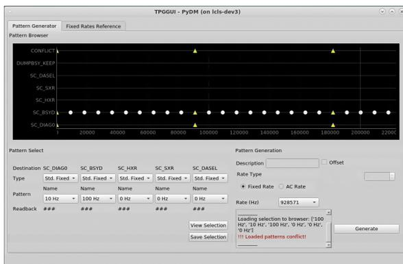
Figure 8: TPGGUI showing conflict on beam pulse requested by SC\_DIAG0 and SC\_BSYD in pulse stealing mode.
