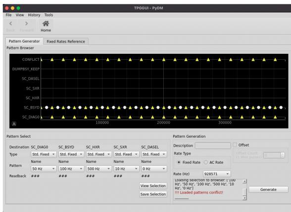
Figure 7: TPGGUI showing conflict on beam pulse requested by two destinations on the same bucket.
