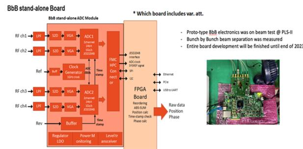
Figure 4: The configuration of BBB BPM electronics.
