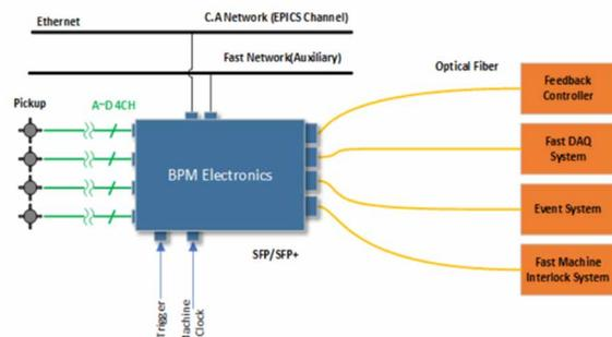
Figure 6: I/O configuration of 4GSR SR BPM electronics.
