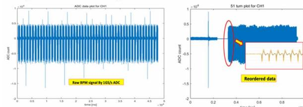
Figure 5: The beam test results of BBB BPM electronics. A signal reconstruction by using BBB signal with 51 turn data at PLS-II storage ring.
