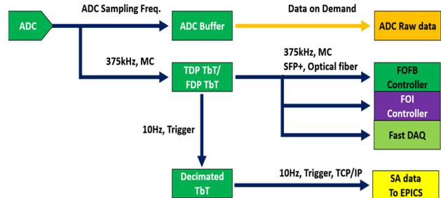
Figure 7: The data flow of 4GSR SR BPM electronics.
