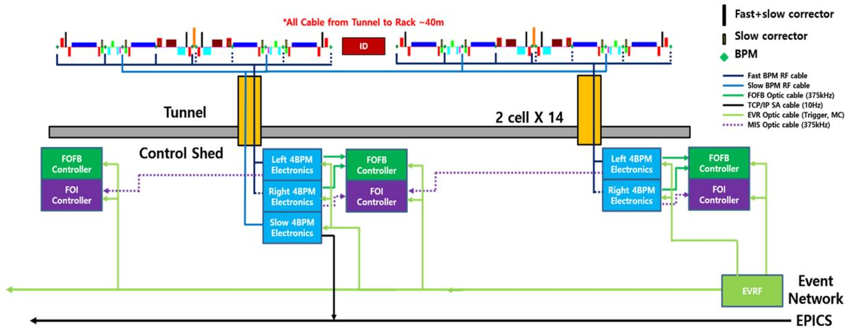
Figure 8: The configuration of BPM RF & timing cable connections for the storage ring.
