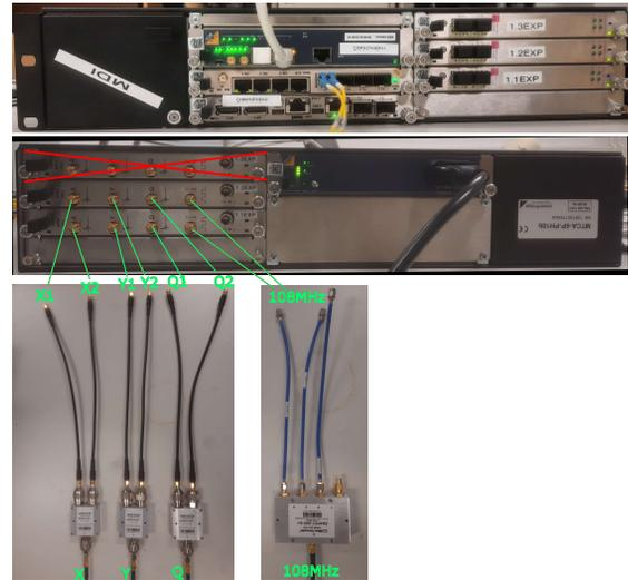
Figure 2: Micro TCA based read-out electronics including CPU, MCH, X2timer, and three digitizer cards. Three power splitters for x,y and q signals from the cavity and an additional splitter for the Master Oscillator reference frequency of 108 MHz.
