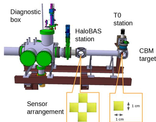
Figure 1: The CBM BMON system consists of two stations for beam halo and T0 measurement. The stations are mounted in standard CF 100 vacuum chambers in front of the CBM target. The T0 station uses a single sensor, while the Halo station uses a mosaic structure of four sensors. The Halo station will also be part of a fast beam abort system (BAS).
