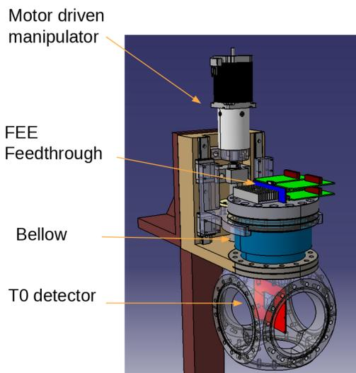
Figure 3: Schematic illustration of the manipulator system for removing the T0 detector from the beam axis.
