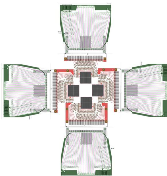
Figure 4: Sensor mount and feed-through PCB. The sensor will be glued into the recess and then bonded to the amplification stage input pads. **Upper panel:** One PCB is needed for the T0 system. **Lower panel:** A mosaic arrangement of four PCBs is used for the halo system.
