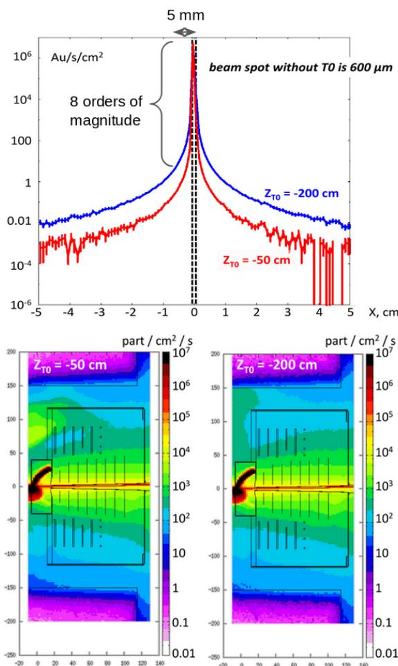
Figure 2: Widening of the beam and charged particle contamination in the STS region for two different T0 positions. **Upper panel:** The widening of the beam due to the diamond material of the T0 detector, which is located 50 cm (red curve) and 200 cm (blue curve) in front of the CBM target. **Lower panel:** The charged particle contamination in the STS region for the two different T0 positions.
