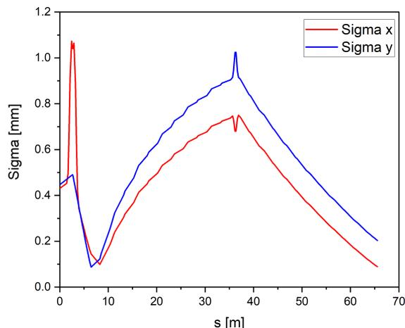
Figure 2: Evolution of the rms beam sizes (horizontal  $x$  and vertical  $y$ ) along the LINAC.
