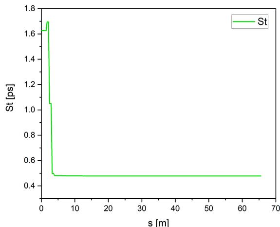
Figure 3: Evolution of the bunch length along the LINAC.
