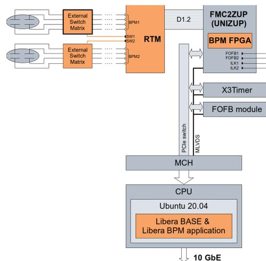
Figure 2: BPM system building blocks and interconnections. Courtesy: I-Tech.
