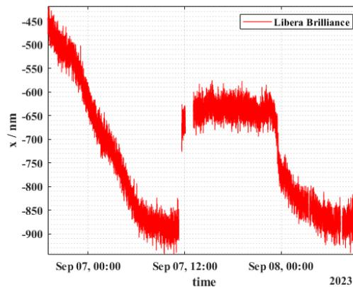
Figure 7: Horizontal position readings acquired from the SA data path with a *Libera Brilliance* under the same conditions as in Fig. 6.
