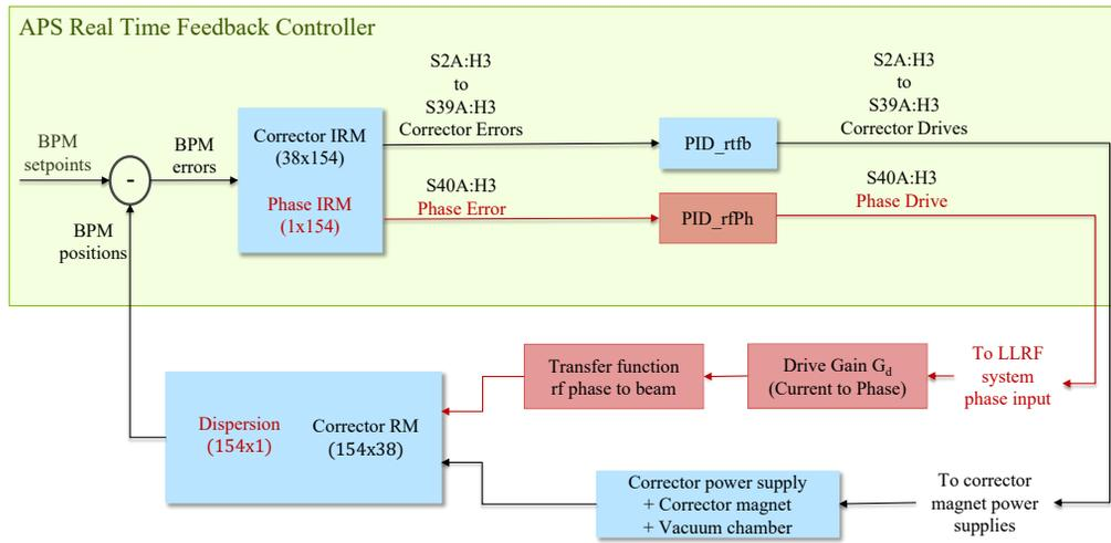
Figure 1: Experimental setup for simultaneous operation of RTFB and orbit to RF phase feedback using APS RTFB system.
