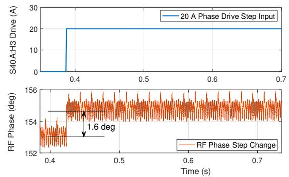
Figure 2: Open loop phase step response measured for 20 A input step amplitude.
