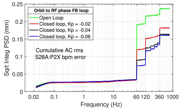
Figure 3: Orbit motion measured in open loop, and closed loop with different proportional gain values.
