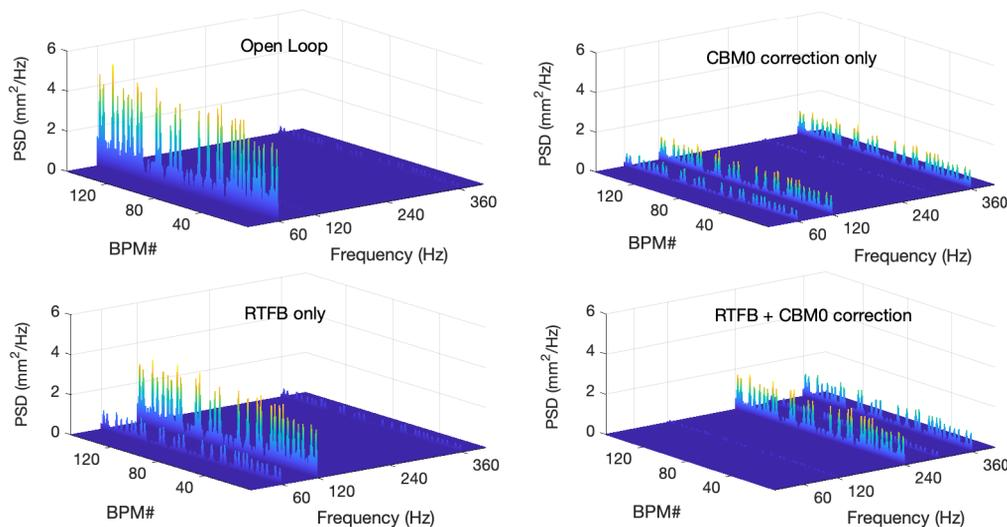
Figure 5: PSD of BPM errors at all 154 BPMs around the storage ring. Comparison of responses in open loop and different closed loop configurations.
