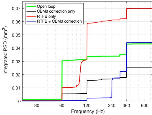
Figure 4: Comparison of cumulative mean square orbit motion at S28A:P2X BPM for different feedback configurations.
