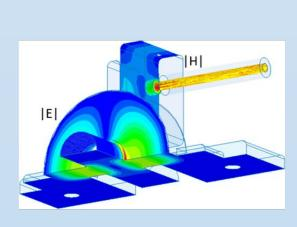
Dipole cavity has two orthogonal coupling slots to selectively measure X and Y position
