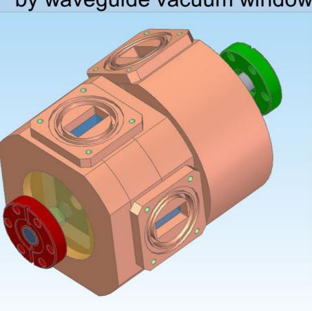
Rectangular dipole cavity and coupling slot machined into solid
