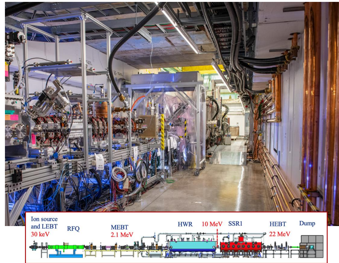
PIP2IT Accelerator Layout – A near full-scale Front- End of PIP-II with first two cryomodules
