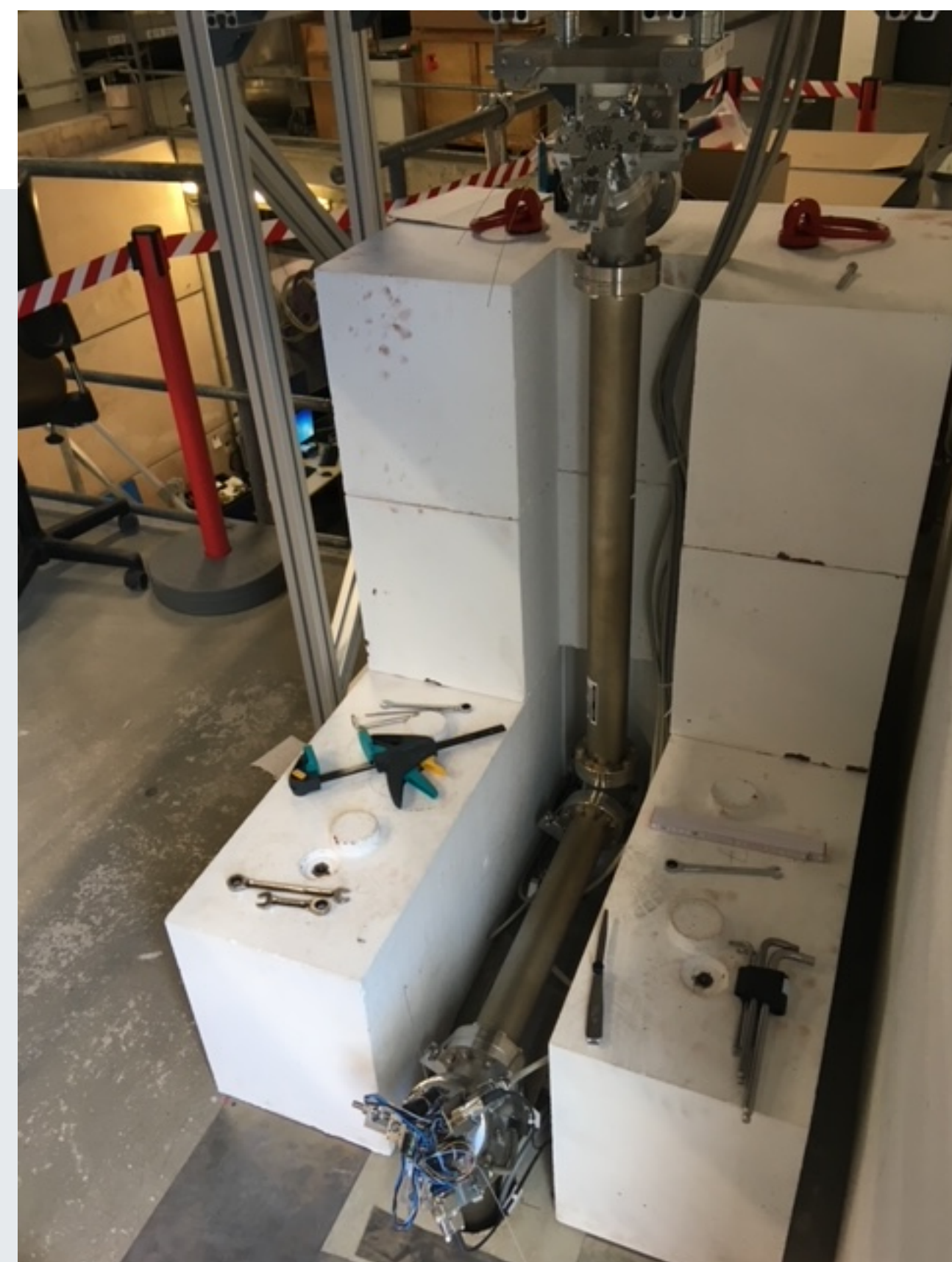
HZB Mirror holder with motorized 2-point tilt adjustment for alignment through the labyrinth.
