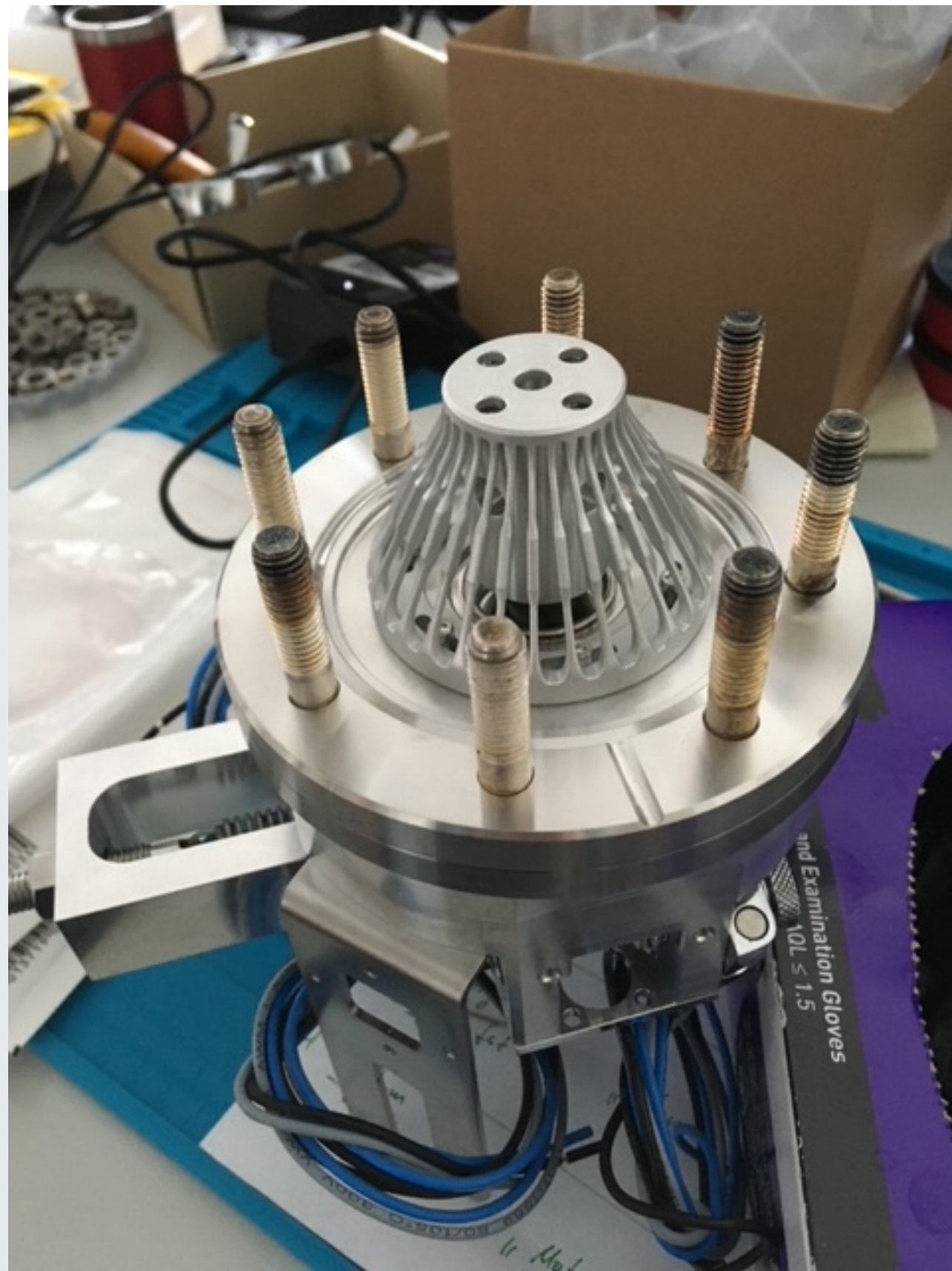
HZB Mirror holder with motorized 2-point tilt adjustment for alignment through the labyrinth.
