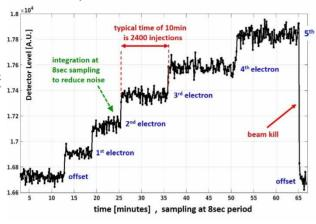
Figure 9: The injection of 1-2-3-4-5 electrons over a time span of 1 hour, measured with 8 sec integration mode.
