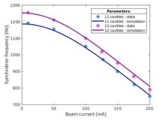
Figure 6: Simulation and measurement results of the synchrotron frequency as a function of beam current.
