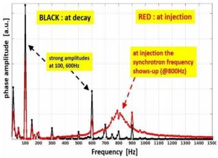
Figure 5: Frequency spectra of the phase, both at injection (red) and during normal decay (black).
