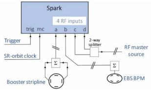
Figure 1: The connections of the phase-monitor.
