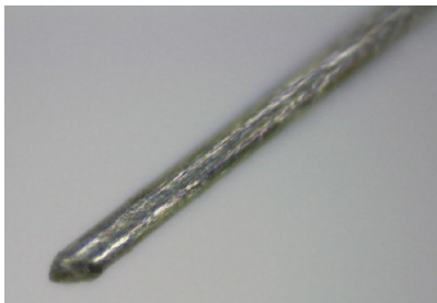
Figure 6: End of broken wire at a magnification of \sim 800 . No thinning is visible.
