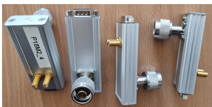
Figure 2: Picture of the head amplifier developed for the HESR BPM system. The N-type plug is main signal input, calibration ports and signal output ports are facilitated via SMA connectors. The power is connected through the D-Sub plug.
