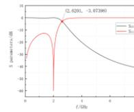
Fig. 2. S parameters of low pass filter
