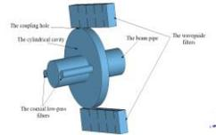
Fig. 5. structure of bunch length monitor
