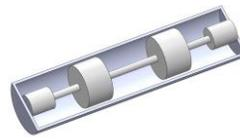
Fig. 1. Structure of low pass filter
