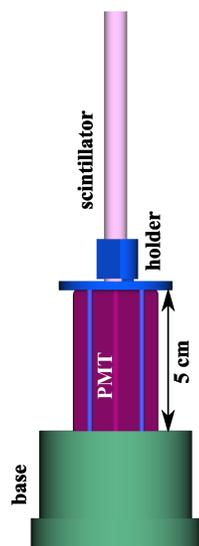
Design of BLM detector for PoFEL accelerator
