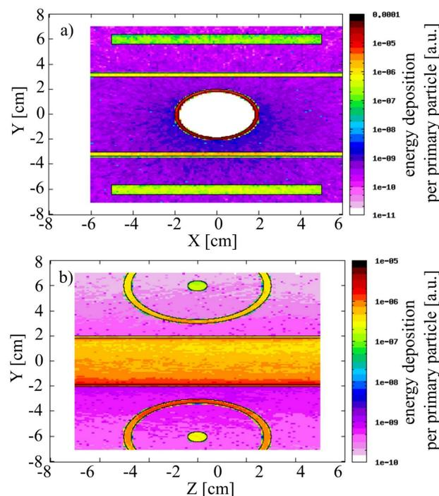
Geometry used during MC simulations (upper left, not to scale) and results of calculations: Energy deposition spectrum (lower left), Energy deposition in Cartesian grid: XY plane (upper right), YZ plane (lower right), as calculated for one of the geometry and chosen detector.
