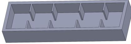
Figure 3: 3D model of band pass filter.
