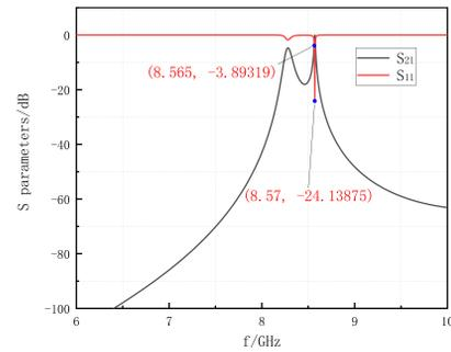
Figure 5: S parameters of band pass filter.
