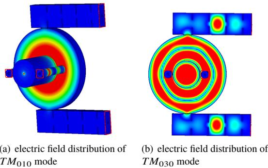
Figure 7: Electric field distribution of coupling mode.
