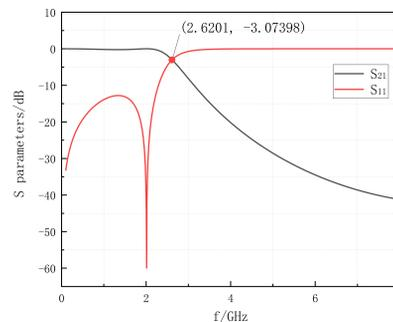
Figure 2: S parameters of low pass filter.
