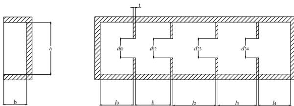
Figure 4: Cutaway view of band pass filter.
