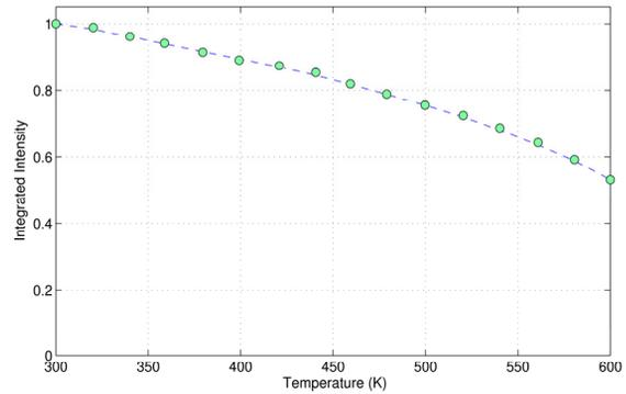
Figure 4: The temperature dependence of YAG yield [3, 6].
