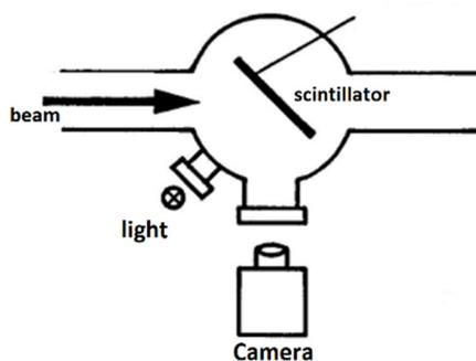
Figure 1: Layout of beam profile diagnostic system.
