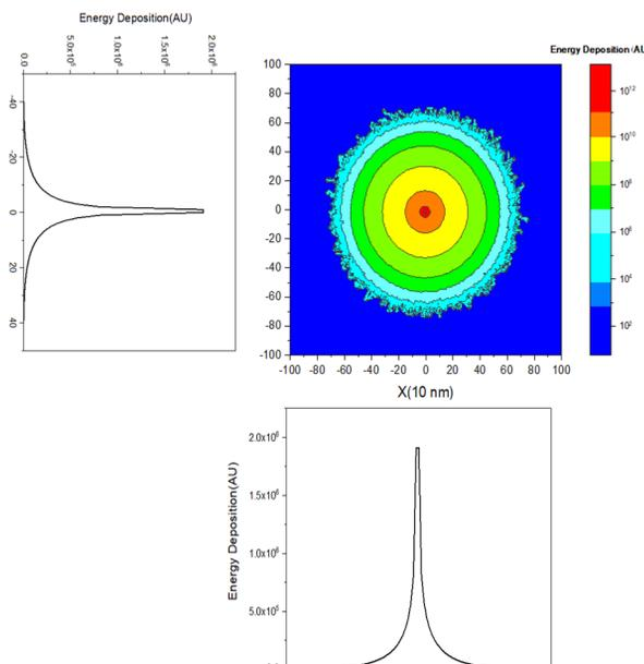
Figure 12: The profile of the 200keV proton beam on the YAG scintillation target.
