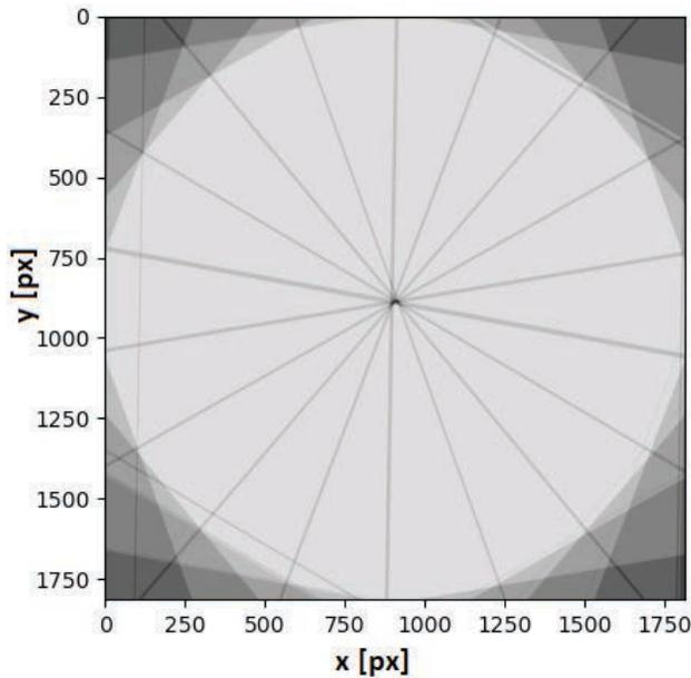
Figure 9: Tomographic reconstruction of the calibration wire from Fig. 4.
