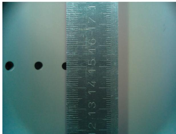
Figure 3: This ruler, which was placed in the center of the beam path at a distance of 0.5 mm, was used for scaling.
