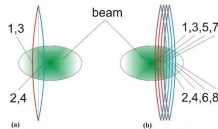
Figure 4: For odd indices the wire at its leftmost position, and for even indices the wire at its rightmost position: (a) the scanner is stationary; (b) the scanner is moving.
