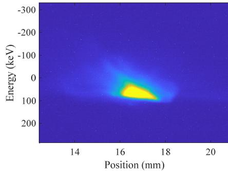
Figure 6: Beam image from the YAG:Ce screen of the spectrometer camera. The image is saturated, but the uncorrelated energy spread can be seen to be <50 KeV.
