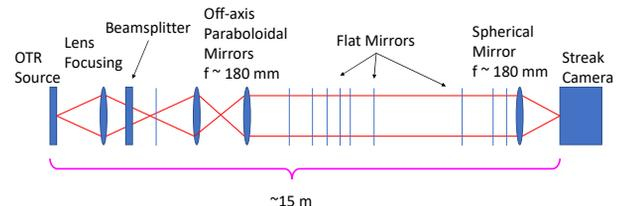
Figure 4: Effective optical path of the new transport line from OTR source, to streak camera (not to scale). There are 10 flat mirrors (indicated by the thin lines) in addition to the labeled optical components.
