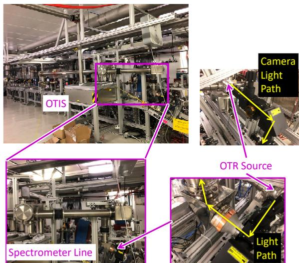
Figure 3: Pictures showing the new optical transport line from the spectrometer camera source point. The yellow arrows show the beginning light path for the new transport line and the spectrometer camera.
