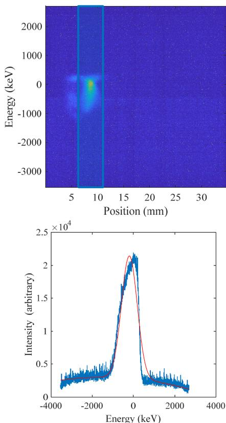
Figure 9: Top) Spectrometer camera image of beam with 15-degree rf phase offset. Bottom) The energy spread projection within the boxed region of interest and a gaussian fit with sigma of 383 KeV.
