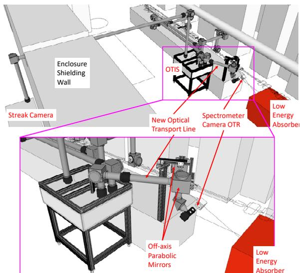
Figure 2: Overview the Optical and Terahertz Instrumentation System (OTIS). The new transport line originates from the spectrometer camera.
