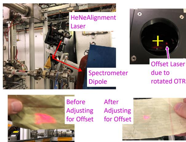
Figure 5: Alignment of the transport line is via a HeNe laser injected through a viewport before the spectrometer magnet. The before and after pictures show the distortion induced by the rotated OTR screen. The yellow cross is the ideal laser position.
