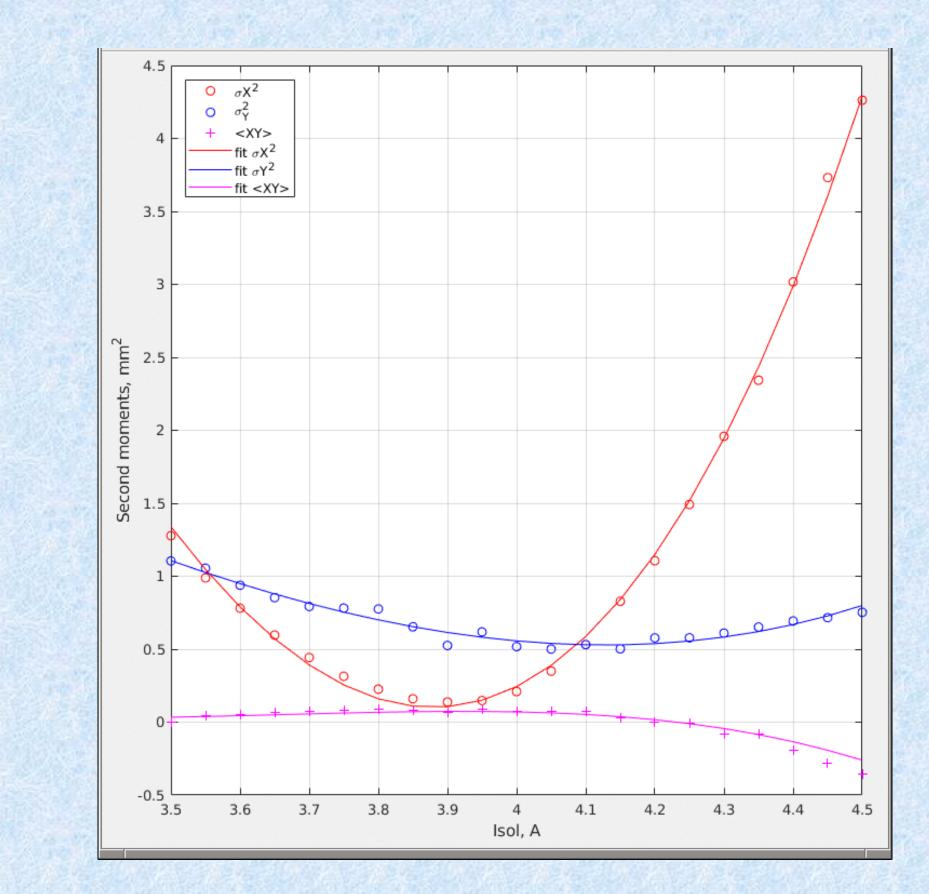
Measurement of the second moments of the 1.6 MeV electron beam distribution in the LeREC accelerator (0.2 A peak current) with solenoid and screen placed 0.76 m downstream. The found second moments are:  $\langle x^2 \rangle = 27.2 \text{ mm}^2$ , <xx'>=0.81 mm mrad, <x'2>=0.03 mrad2, <y<sup>2</sup>>=6.1 mm<sup>2</sup>, <yy'>=0.32 mm mrad, <y'2>=0.05 mrad<sup>2</sup>, <xy>=6.0 mm<sup>2</sup>, <x'y'>=0.0 mrad<sup>2</sup>, <x'y>=<xy'>=0.13 mm mrad.
