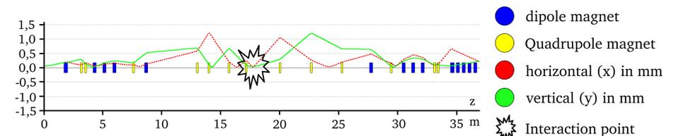
Preliminary electron beam simulation at interaction point. Beam envelope ( $1\sigma$ ) simulation at third recirculation. Beam focuses at interaction point.
