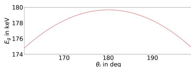
$y$  energy of inverse Compton scattering for 1.2 eV incident photons over the angle between laser and electron beam at 98.8 MeV.
