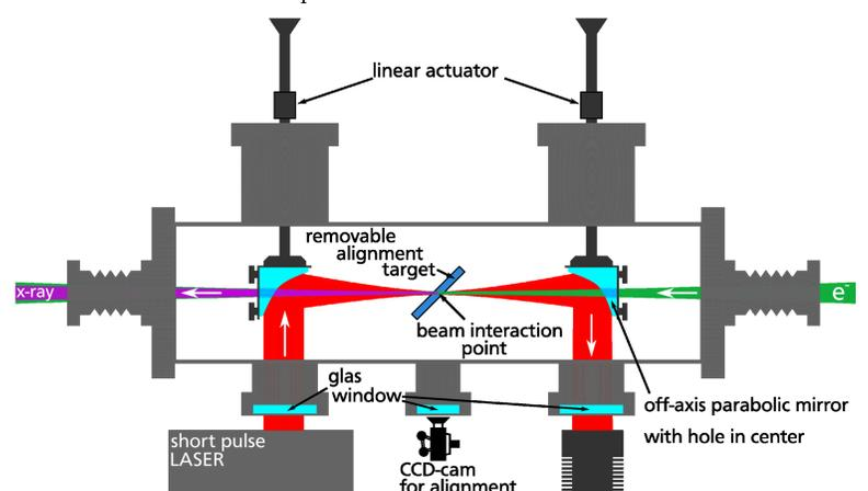
Preliminary design of the chamber located at the interaction point in the third recirculation. Concept adapted from [5].
