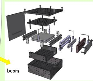
Detailed view of different parts of probe. Heat will be deposited on entrance slit and transferred by conduction and radiation to cooling screen and other parts
