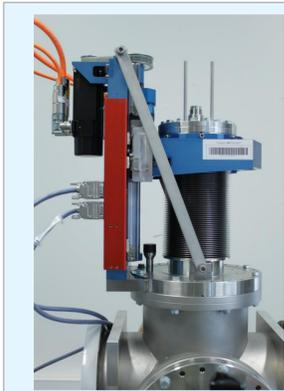
Transverse phase space scanner enables emittance measurement for low energy ion beams. It is a slit-slit system based on Allison principle and has an electrostatic deflector, an electron repeller and a Faraday cup. The electronics and data processing is mainly based on CompactRio and Labview standards
