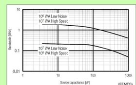
Measurement of bandwidth and frequency linearity of current-voltage convertor. Specific case for low current < 50 nA. BW increases with intensity and decreases with charge capacitance (~ 100 pF for real case with coax cable)
