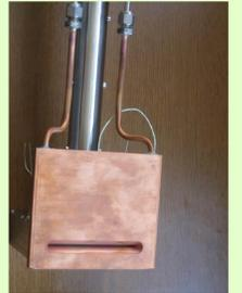
Cooling screen with entrance slit, water circuit and feedthroughs
