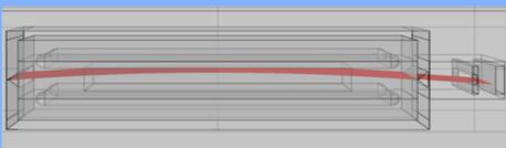
Trajectory of ions without and with losses. Study case : 60 keV beam emission with 80 mrad incidence and ± 760 V deflecting voltage
