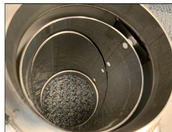
Figure 3: Picture of split-plate BPM implemented.
