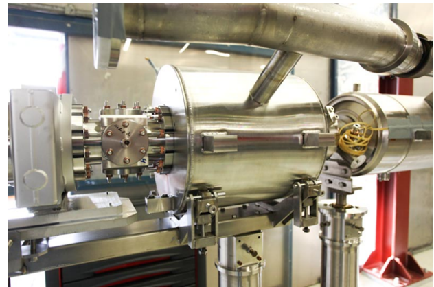
Figure 2: Photo of components at the end of a cryogenic module before installation; from right: housing of the cavity, housing of the quadrupole, button BPM.
