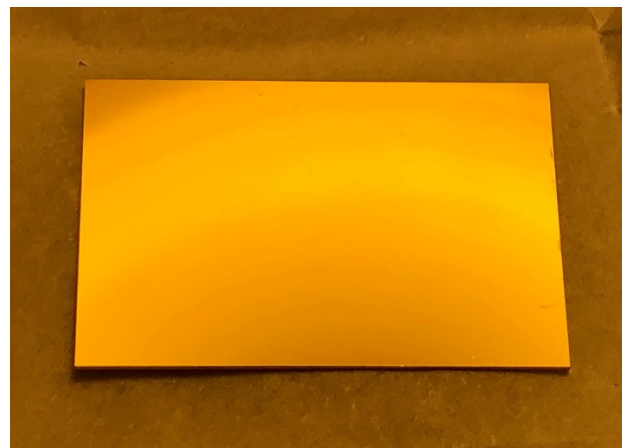
Figure 1: A 20 mm x 30 mm x 0.5 mm diamond mirror, consisting of six 10 mm x 10 mm monocrystals fused together, with 3 μm Au reflective coating. The light intensity pattern seen on the mirror surface comes from the reflector of the lamp used to illuminate it.
