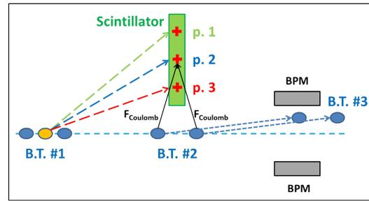
Figure 6: Measurement scheme.
