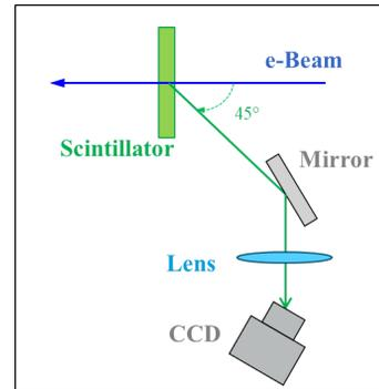
Figure 1: Standard scheme of scintillating screen monitors at the European XFEL.
