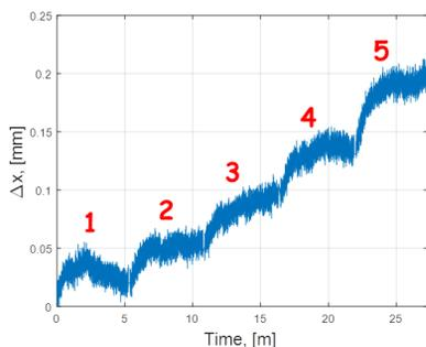
Figure 8: Horizontal bunch deflection as measured with the BPM 4 m downstream the screen monitor. The red numbers correspond to the positions of the bunch onto the screen.
