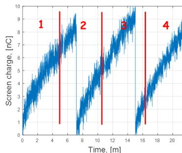
Figure 12: Accumulated screen charge as converted from orbit deflection.
