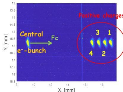
Figure 11: Bunch positions in the second measurement.
