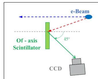
Figure 2: Off-axis screen scheme. Blue line: normal trajectory of electron bunches, red line: bunch trajectory of kicked ones crossing the scintillator.
