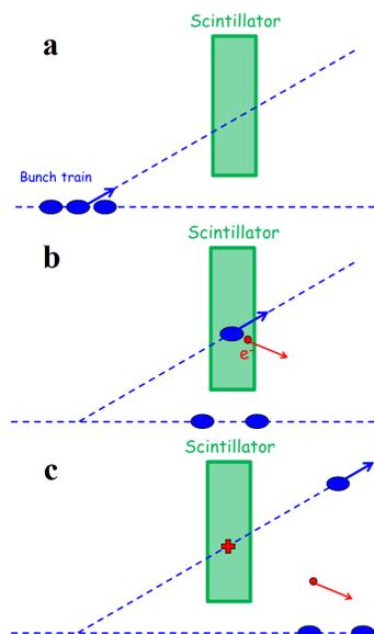
Figure 5: Illustration of the screen charging mechanism.
