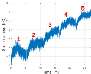
Figure 9: Accumulated screen charge as converted from horizontal bunch deflection in Fig. 8.
