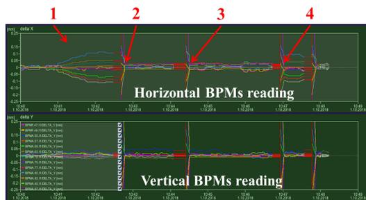
Figure 4: BPMs readings downstream the injector screen stations: 1. an off-axis screen was inserted and a bunch kicked on it; 2. the screen was retracted; 3. another off-axis screen was inserted without kicked bunch; 4. the second screen was retracted and the first one moved back in.
