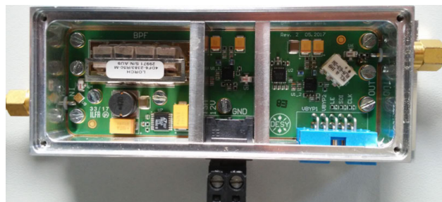
Figure 7: Coarse BAM analog front end.
