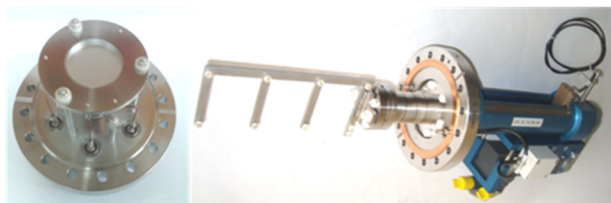
Figure 7: X-ray detector (left) and mechanical system for wire insertion (right) of BEM.
