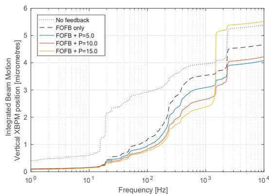
Figure 7: The measured integrated X-ray beam motion as the SOFFOX proportional gain is increased. The nominal stability of the X-ray beam with FOFB running is shown by the dashed black line.
