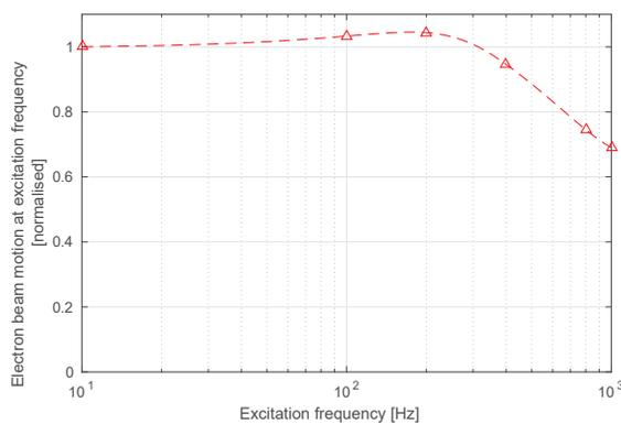
Figure 3: The measured electron beam motion as a function of corrector magnet excitation frequency in open-loop.
