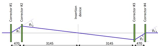
Figure 2: A sketch (not to scale) showing the magnet configuration used to produce a closed bump through the ID straight. Distances given are in millimetres.
