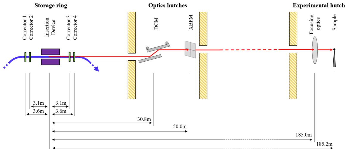
Figure 1: A sketch (not to scale) showing the layout of the I14 beamline and the location of the four SOFFOX chicane magnets.
