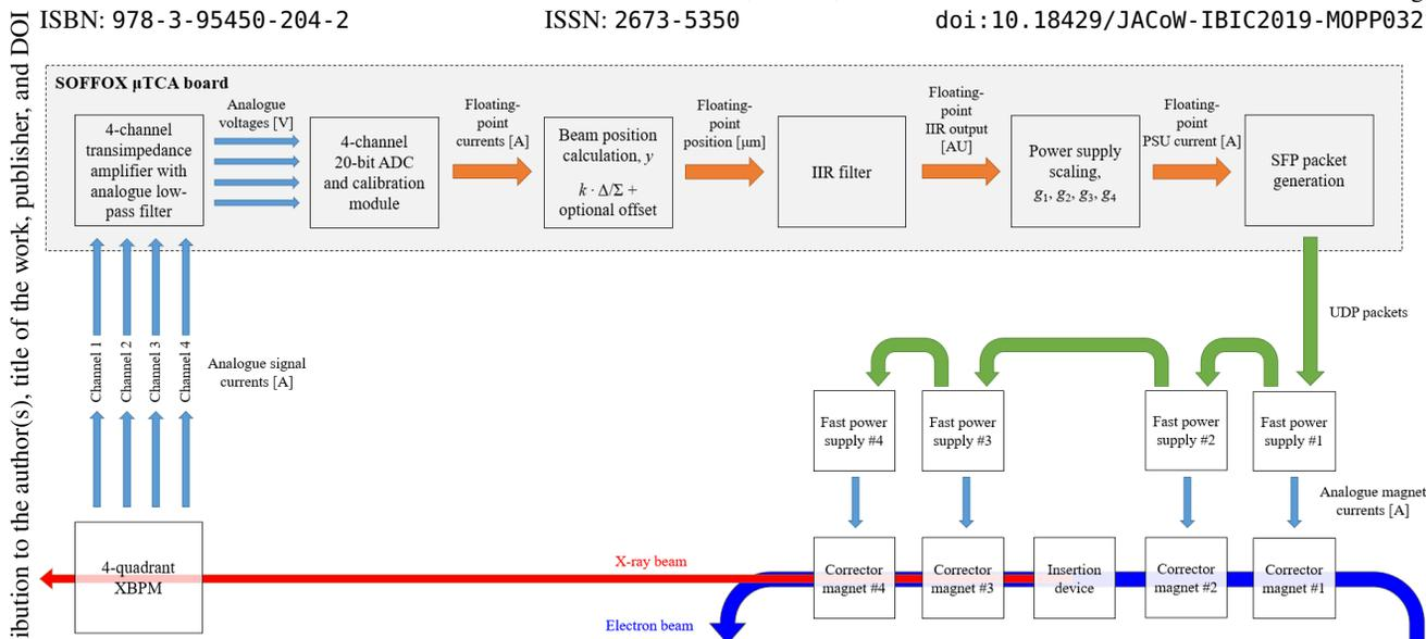
Figure 4: A block diagram showing the processes involved in the SOFFOX feedback scheme.
