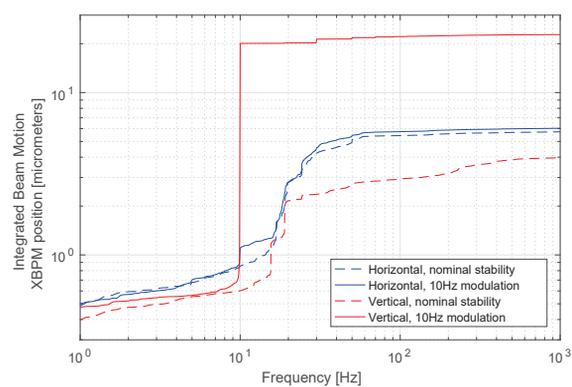
Figure 6: There is a small additional 10 Hz component visible in the horizontal beam motion whilst the system is applying a vertical 10 Hz modulation to the X-ray beam.
