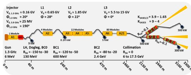
Figure 1: Schematic overview of the European XFEL accelerator [2].
