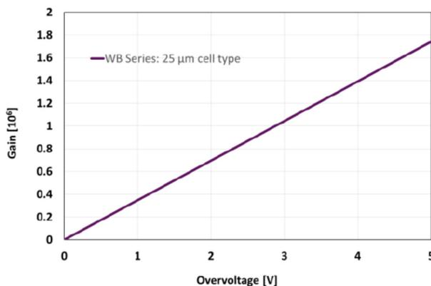
Figure 4: SiPM gain versus bias voltage [3].
