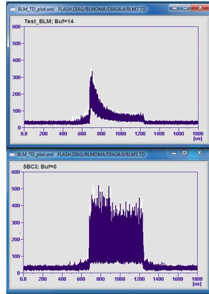
Figure 5: SiPM (top) vs. PMT (down); Darkcurrent signal over pulstrain; SiPM bias voltage drops due to too less bias current.
