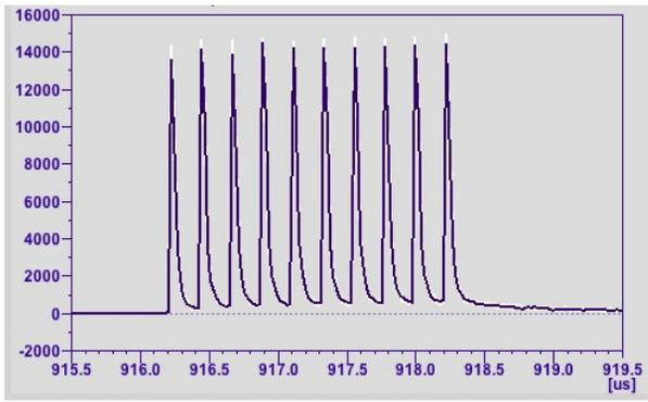
Figure 7: SiPM response, 10 bunches @ 4.5 MHz rep. rate, cherenkov, bias +29V.
