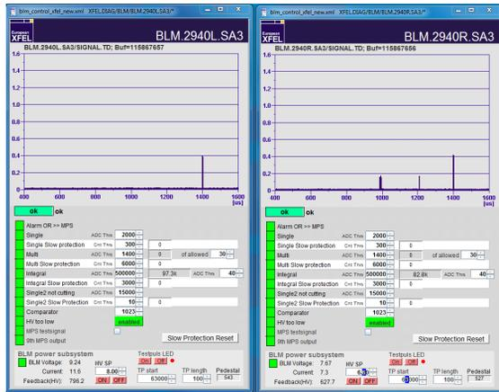
Figure 8: SiPM (left) and PMT (right), no radiator installed, Test LED signal at 1400 us
