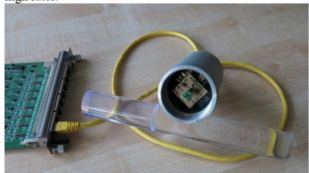
Figure 10: RTM and BLM with SiPM readout (prototype).
