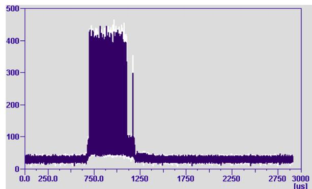
Figure 6: SiPM response, 400 bunches @ 1MHz rep. rate + 1 bunch, scintillator, bias +27V.
