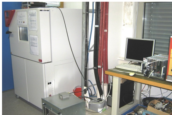
Figure 1: Climate cabinet with dose measurement setup.
