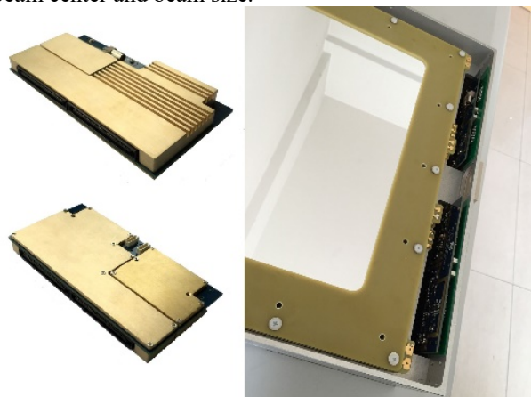
Figure 4: The integrated front-end electronics.
