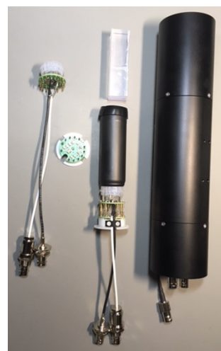
Figure 1: An assembled BLM detector is shown to the right of the photograph. In the middle the scintillator, photomultiplier and voltage divider are shown. A disassembled active voltage divider is placed to the left of the photograph.
