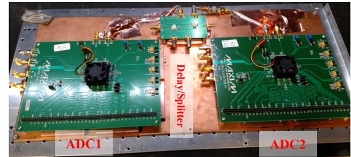
Maxim ADC Eval Boards Mounted to Grounding place
