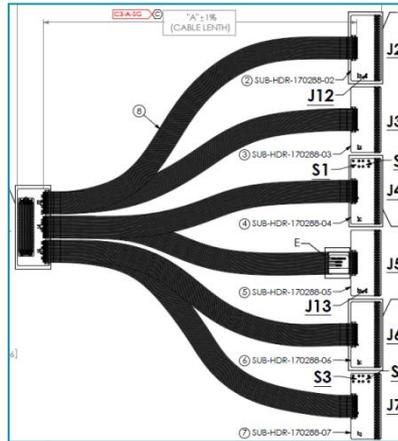
Custom High-Speed ADC Interface Cable Assembly (made by Samtec, Inc.)
