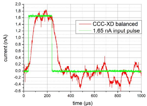
Figure 7: Balanced system response (red) of a low-level  $200 \mu\text{s}$  pulse signal (green), without digital data processing, an analogue 10 kHz low-pass filter is used.
