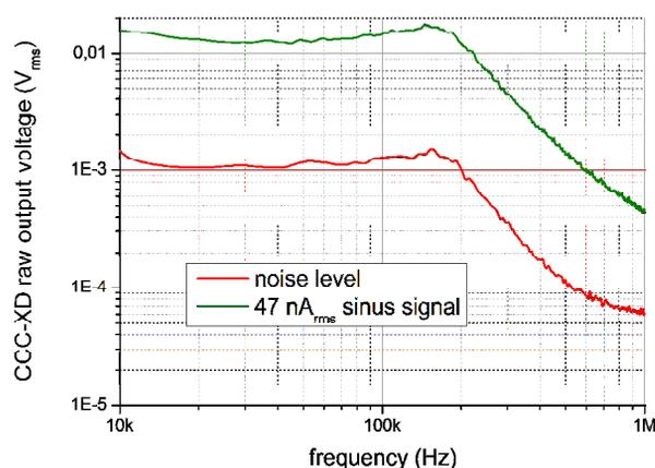
Figure 6: Small-signal response compared to noise level.
