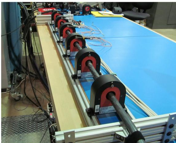
Figure 5: DCCT evaluation with common primary current.
