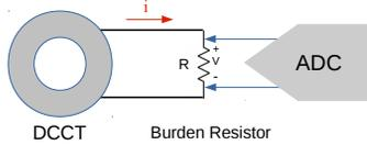
Figure 2: Basic components of a current measurement channel.
