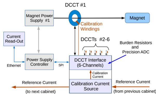
Figure 1: Current measurement and calibration system.
