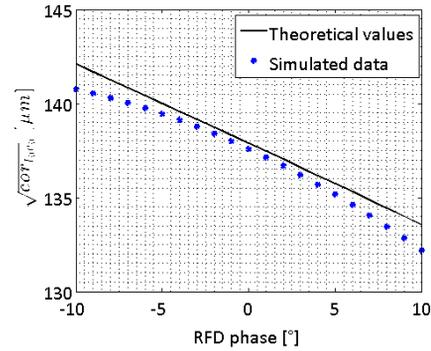
Figure 2:  $\sqrt{cor_{10v0}}$  versus deflecting voltage phase. Simulated data in blue stars (i.e. the square root of the half of the difference of squared vertical spot size measurements at screen with deflecting voltage phase  $\varphi$  and  $\varphi + \pi$ ), and theoretical values (1) in black line.
