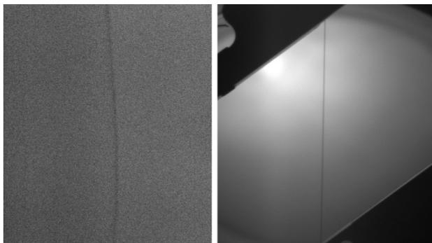
Figure 3: Wire at 3.25 m/s: distorted (left), straight (right).
