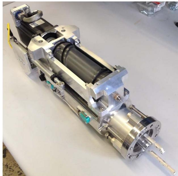
Figure 1: TRIUMF Fast Wire Scanner assembly.
