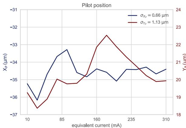
Figure 8: Constant amplitude at ADCs input: pilot position during an equivalent current ramp of 10-310 mA.
