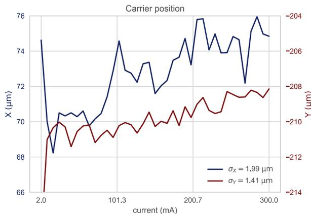
Figure 4: Beam position during a current ramp.
