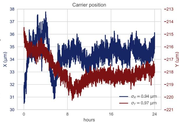
Figure 3: Beam position in a time window of 24 hours.
