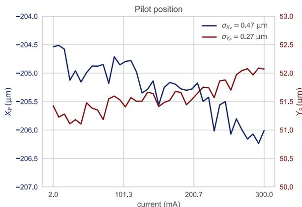
Figure 5: Pilot position during a current ramp.
