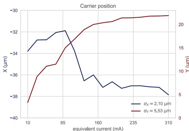
Figure 6: Carrier position during an equivalent current ramp of 10-310 mA.
