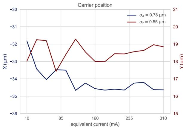
Figure 7: Constant amplitude at ADCs input: carrier position during an equivalent current ramp of 10-310 mA.
