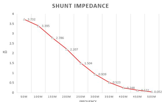
Figure 1: The shunt impedance at different frequencies.
