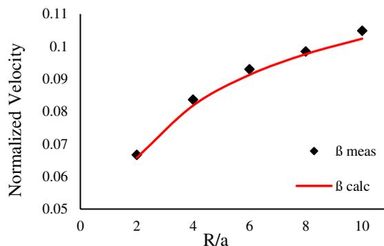
Figure 2: Velocity comparison for different ratios of pipe radii,  $R$ , to helix radius,  $a$ . Sheath helix phase velocity of 0<sup>th</sup> mode in red and results of simulations in black.
