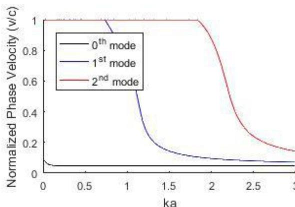
Figure 1: Normalized phase velocity of the first three modes of a sheath helix, pitch angle is 0.048 rad and  $R/a=4$ .  $k$  is the free space propagation constant and  $a$  is the helix radius.
