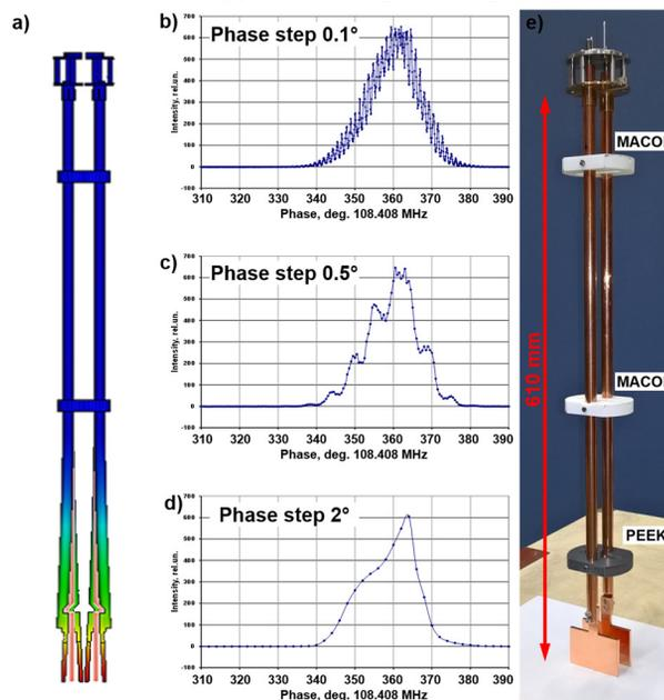
Figure 7: a) Simulated main eigenmode of the electrodes oscillations in a  $\lambda/4$ -type deflector. b-d) Experimental main bunch shape measurements in the presence of vibrations. e) Photo of the RF-deflector with extra PEEK holder.
