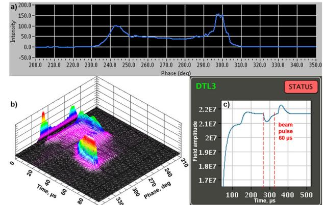
Figure 10: Experimental data from LINAC4 CERN. a) A bunch shape with  $1^\circ$  resolution. b) Evolution of a bunch shape during a beam pulse. c) Behaviour of the field amplitude in DTL3 in the presence of the beam.
