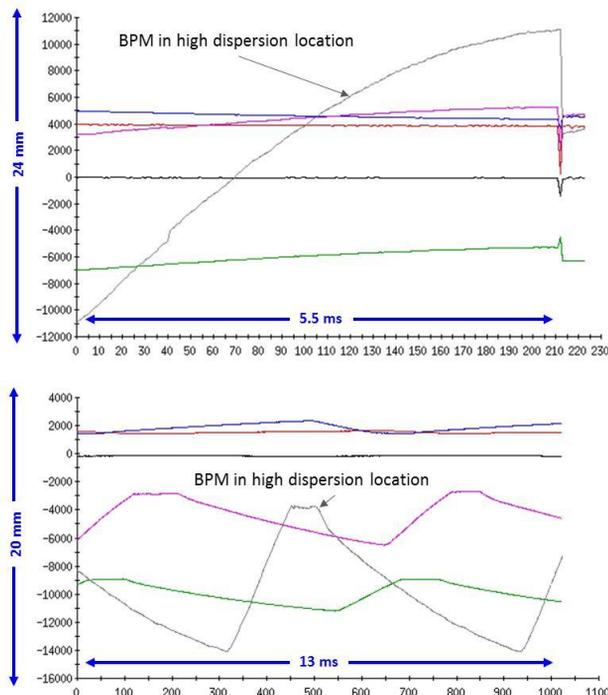
Figure 8: BPMs readings when the beam loading is happening along the train of 50000 MBs with 60 pC/MB (upper plot) and when the gun HVPS regulation loop is malfunctioning in CW mode at 2.8 mA current (lower plot).
