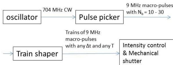
Figure 2: Laser pulse shaping scheme.
